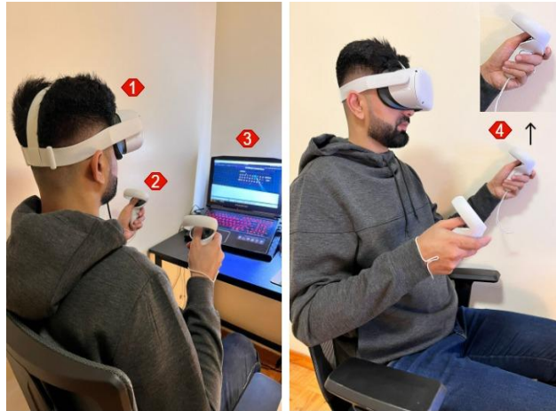
Figure 4: Setup. (1) User wearing Meta Quest 2 HMD, (2) Meta touch controllers, (3) optional PC connected to Meta HMD, (4) user clicks trigger to select a letter from virtual keyboard.
