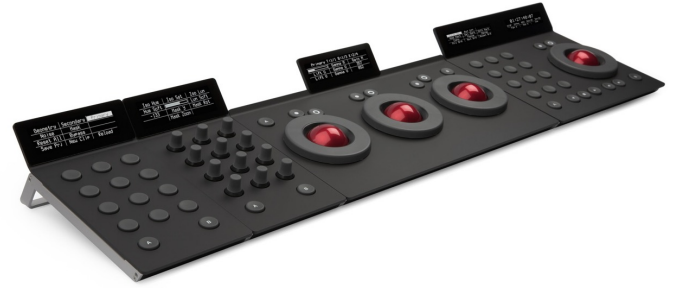
Figure 7: Tangent Element color correction interface (tangent-wave.co.uk). Trackballs are heavily used in cinema and television color correction.
