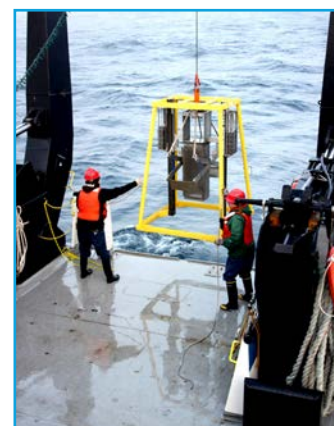
RETRIEVAL OF THE BOX CORER CONTAINING LAKE ERIE SEDIMENTS, FROM WHICH THE SEDIMENT CORES WERE RETRIEVED FOR THIS STUDY. PHOTO COURTESY OF EUAN REAVIE AND DMITRI PERLOV
